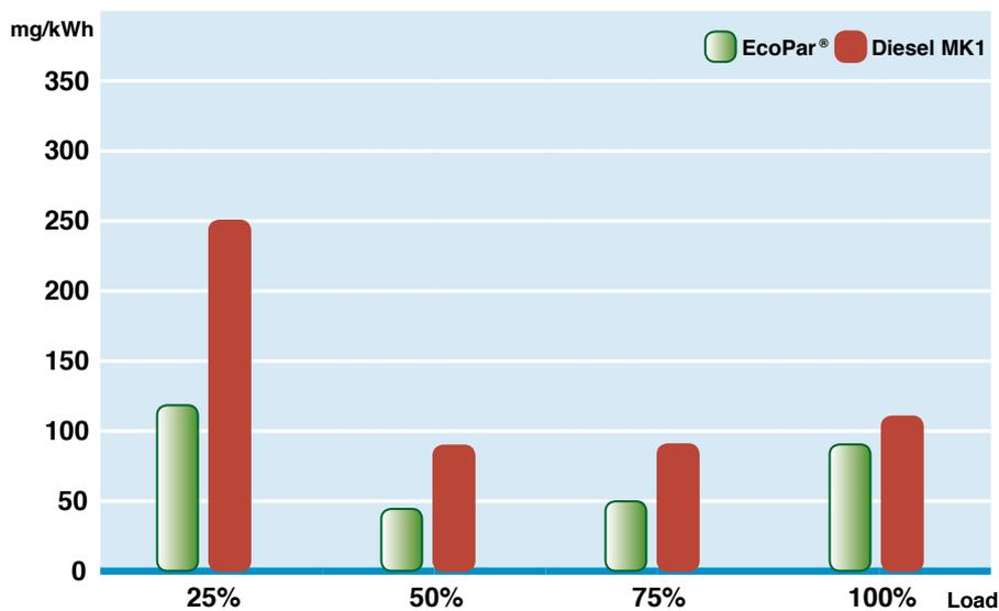
*Emission of soot from a heavy engine with particle trap (DNOx) and ERG (Emission Gas Recycling). Measurements performed by STT Emtec, Sundsvall. "Diesel MK1" is the Swedish Ultralow sulphur diesel (less than 10 ppm sulphur).*
